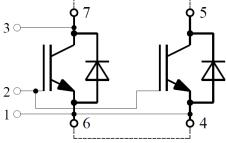
external connection to be done Equivalent Circuit Schematic
